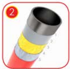
2 Solid construction made of black steel S235JR, cleaned in the sandblasting process. Protected against corrosion by galvanizing and powder coating with polyester paint QUALICOAT attested. 1 - steel, 2 - sandblasting, 3 - iron phosphatizing, 4 - zinc base, 5 - polyester powder paint.
