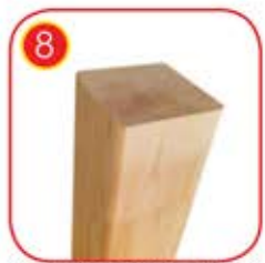
8 Soft conifer wood 90 x 90 mm, coreless, glued in layers with polyurethane glues, totally resistant to water. Wood posts processed in three-phased impregnation process.
