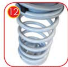
12 Springers' springs made of spring steel. The diameter of the spring is 200 mm and the diameter of the rod is 20 mm. The springs and the fastenings are galvanized and powder coated with polyester paint, UV resistant and QUALICOAT attested. The fastenings are designed especially for solutions used on a playground, so they are stripped of elements which can cause danger to children.
